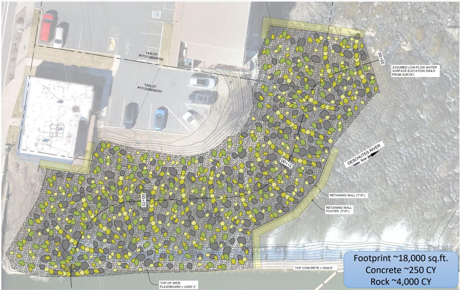
1 ROUGHENED CHANNEL PLAN VIEW 1" = 20'
