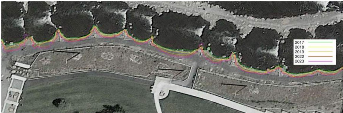
Figure 34. Left bank line degradation over time based on Google Earth aerial imagery. Base photo 2017 from Google Earth.
